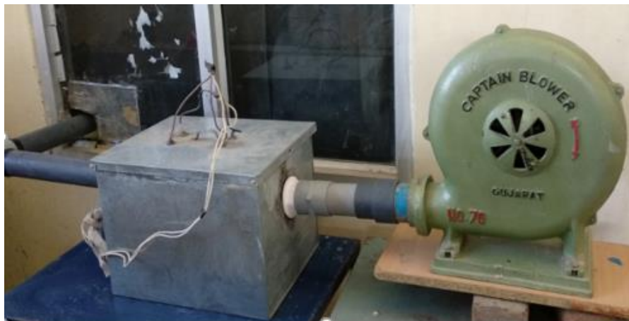
Fig. 3 Centrifugal blower and Air-heater
